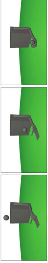
Fig. 4. Visualization of the simulated robot hand while catching a ball. The ball is released 5 units above the palm, where the palm dimensions are 1 \times 0.1 \times 1 units. When the fingers grasp the ball and do not release it throughout the episode, the best possible return (close to -1.0 ) is achieved.
